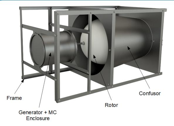
Your SETUR-L bladeless turbine is an environmentally friendly device that uses vortex phenomenon to harness the kinetic energy of water flow in order to produce electricity. SETUR turbine can be cost-effectively used as a standalone self-contained system or in multi-unit hydropower farms.
